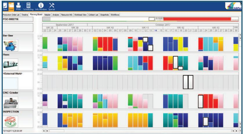
By scheduling a potential job in test mode, you can see where it will fit into your current mix and move it around the Planning Board to uncover possible conflicts with existing job timelines, machine assignments, and material needs.
