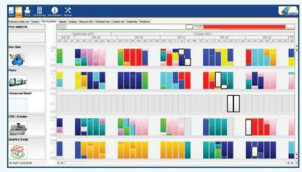
By scheduling a potential job in test mode, you can see where it will fit into your current mix and move it around the Planning Board to uncover possible conflicts with existing job timelines, machine assignments, and material needs.
