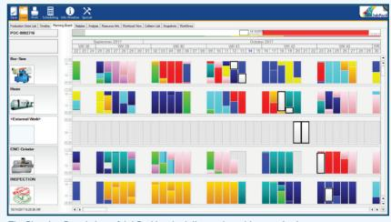
The Planning Board view of JobPack's scheduling and machine monitoring software can help you see the adjustments you need to make to machine and staffing levels, based on all movements in the schedule.
